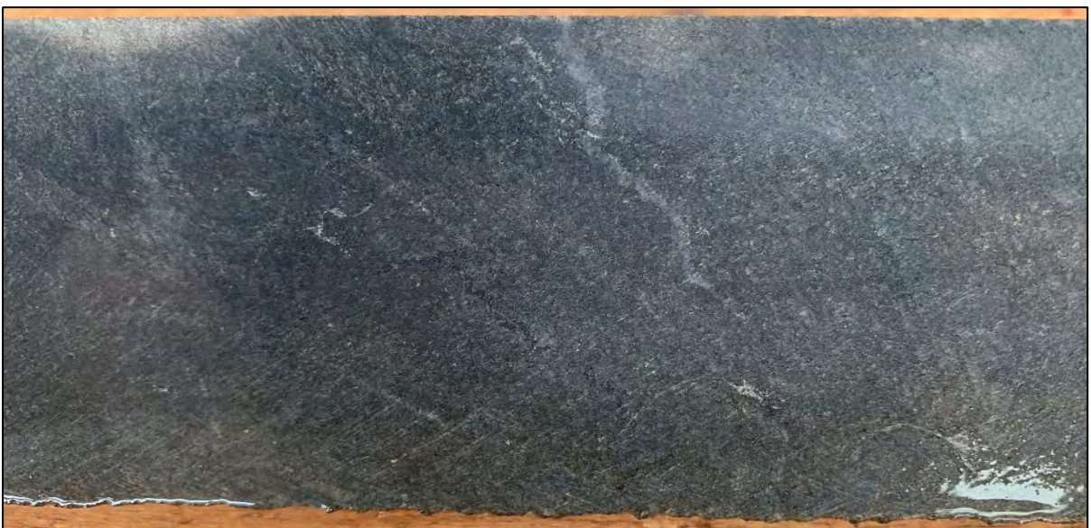
BSD from MRRD001 at 227.3m depth with deformed VQS present in the left of the photo Source: Montage
