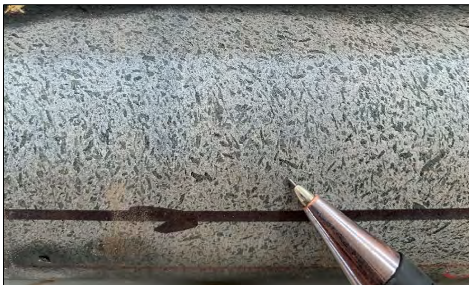
Example of IDY displaying randomly orientated amphibole in MDD010 at 184m depth Source: Montage
