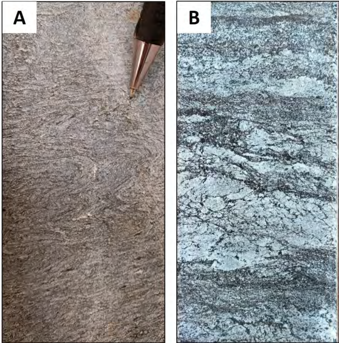
Figure 7-16 Ductile shear within diorite
