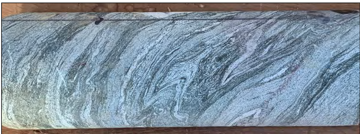
Example of ductile folding within the mafic volcanic unit due to the footwall shear zone (MDD038, 232.8m, 0.04g/t) Source: Montage
