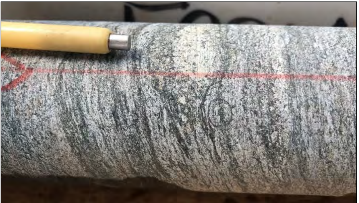
VC1 from MRRD001 at 63m depth. Note the large clast in the center of the photograph with the foliation of the rock wrapping around it Source: Montage.
